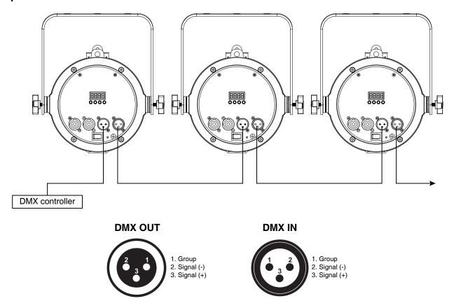
If you are using controllers with this occupation, you can connect the DMX-output of the controller directly with the DMX-input of the first fixture in the DMX-chain. If you wish to connect DMX-controllers with other XLR-outputs, you need to use adapter-cables.
