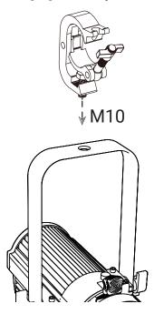
any other orientation, you must use a half-coupler clamp that completely encircles the truss chord.
